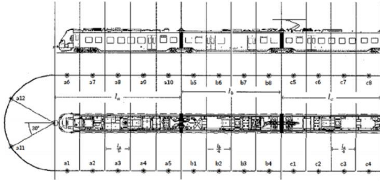
Figure 7 – Example of a mesh of measurement positions for noise level evaluation
